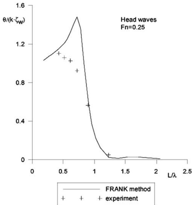
Figure 6 Non-dimensional transfer functions of pitch motion in regular head waves
