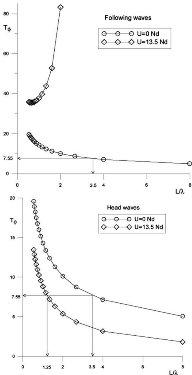
Figure 4 The necessary conditions for induced roll motions in the second instability domain (main resonance)
