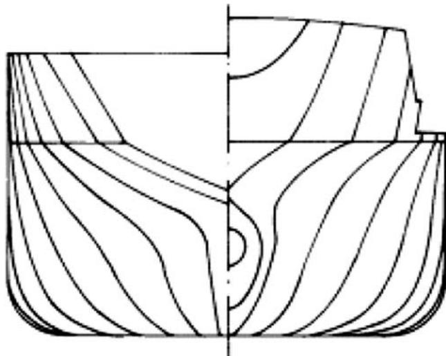
Figure 1 The body plan of the cargo ship
