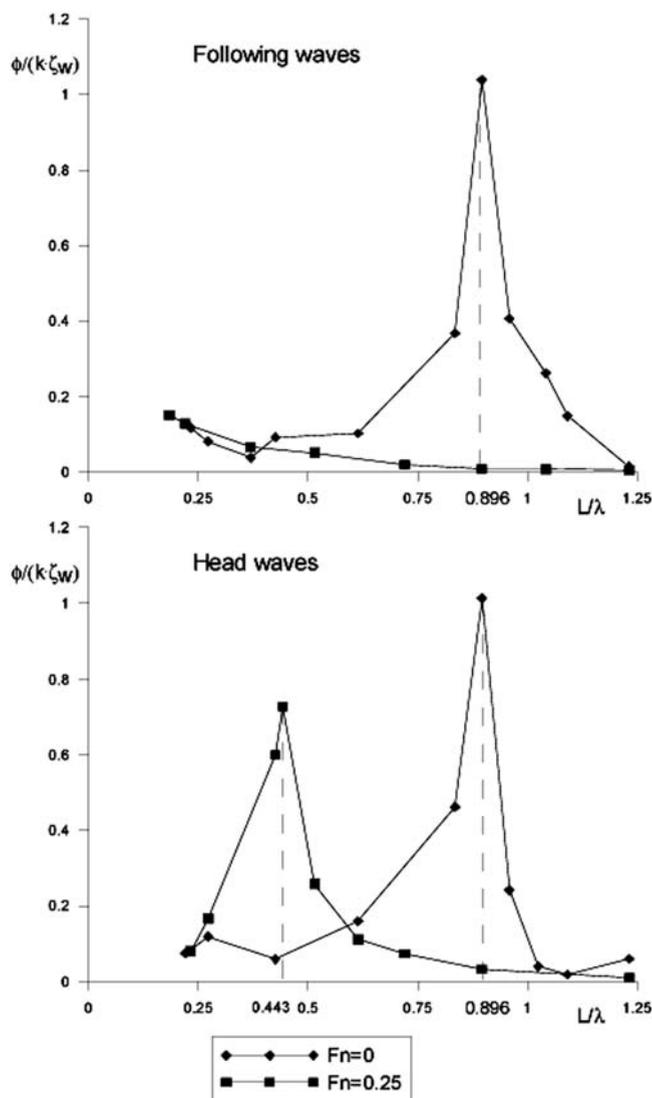
Figure 9 Non-dimensional transfer functions of induced roll motion in regular longitudinal waves
