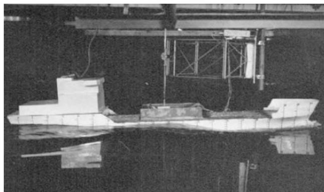
the amplitude of the excitation moment at induced rolling is a linear function depending on the heeling angle
