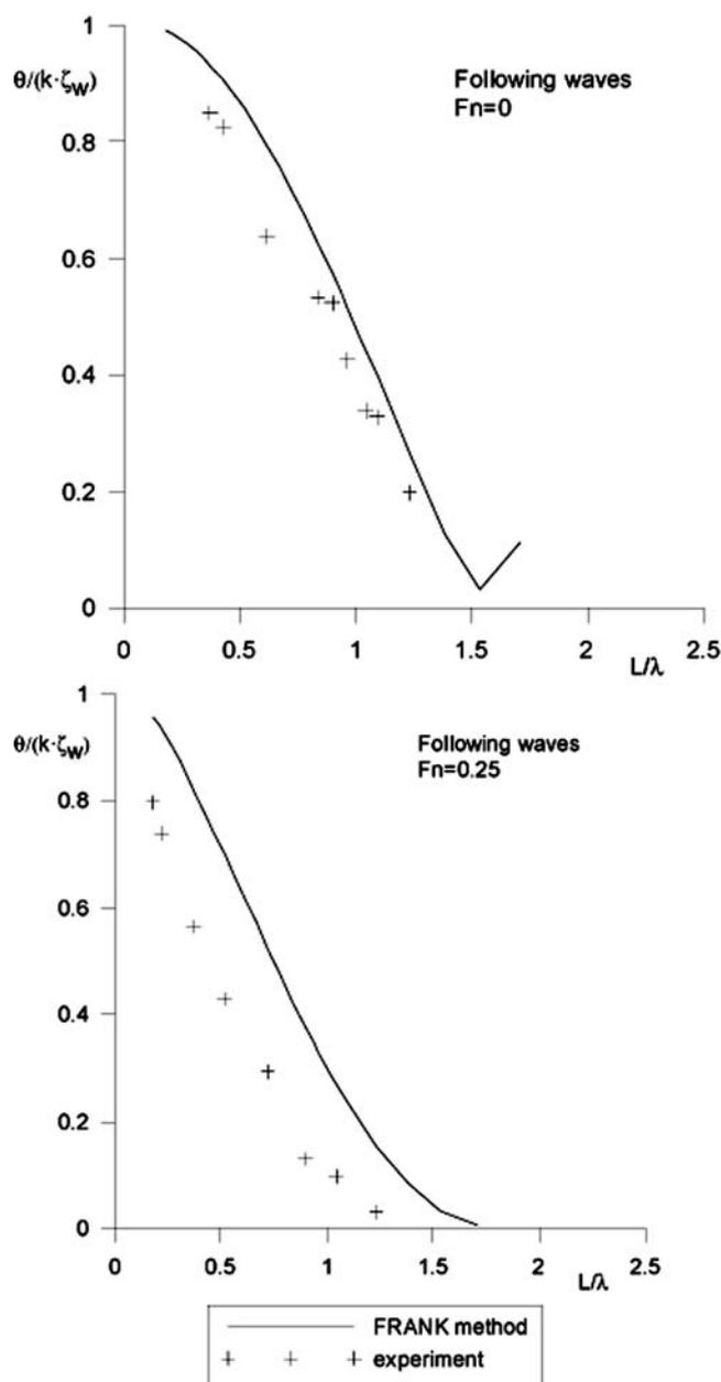
Figure 8 Non-dimensional transfer functions of pitch motion in regular following waves
