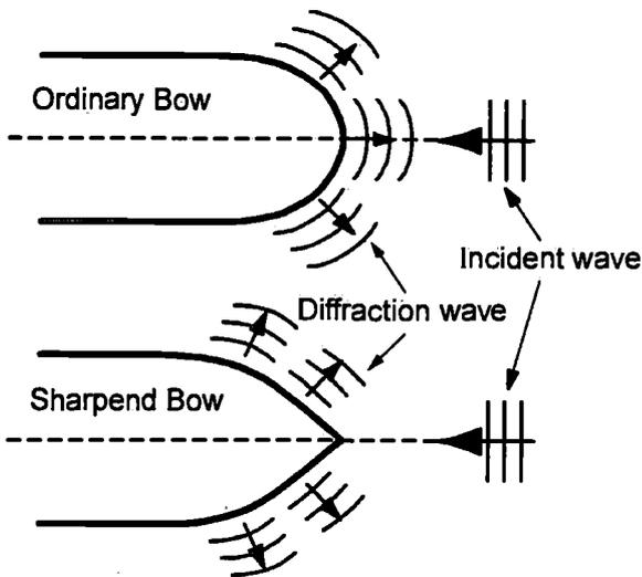
Fig.2 Wave Reflection at Bow
