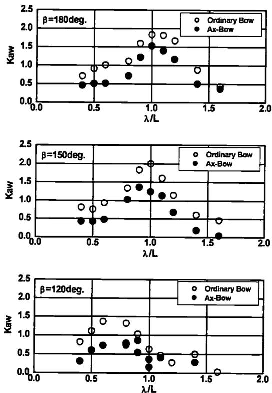
Fig.9 Added Resistance Coefficient for Ax-Bow from Model Test
