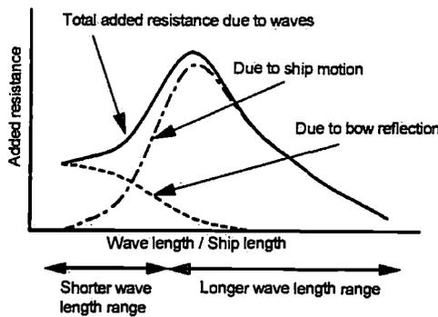
Fig.1 Components of Added Resistance due to Waves
