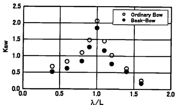
Fig.7 Added Resistance Coefficient for Beak-Bow from Model Test
