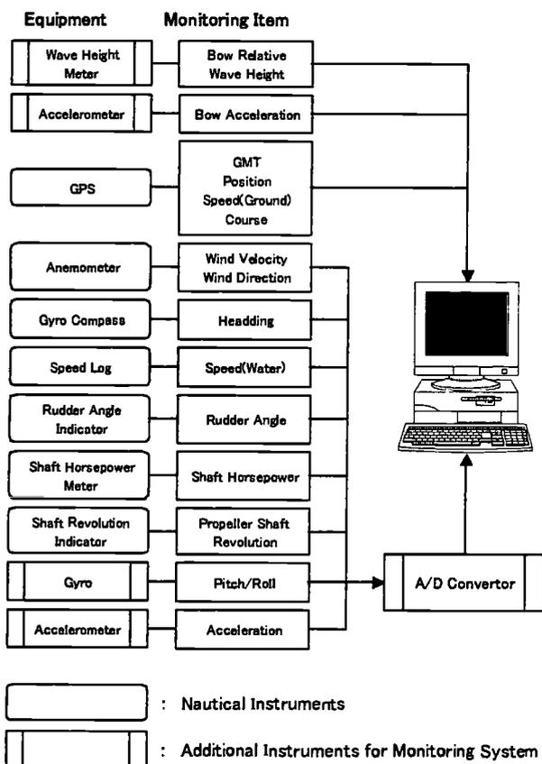
Fig.14 Hull Performance Monitoring System
