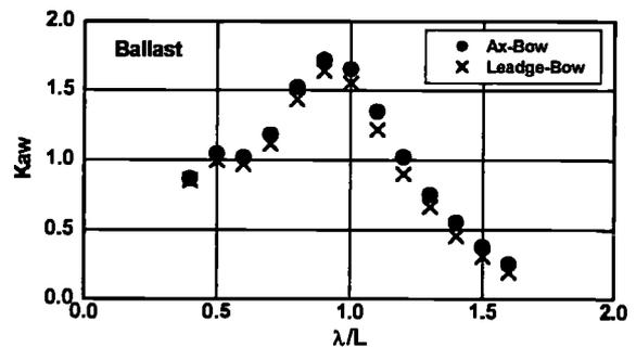
Fig.12 Added Resistance Coefficient for LEADGE-Bow from Model Test (Ballast)
