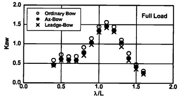
Fig.11 Added Resistance Coefficient for LEADGE-Bow from Model Test (Full Load)
