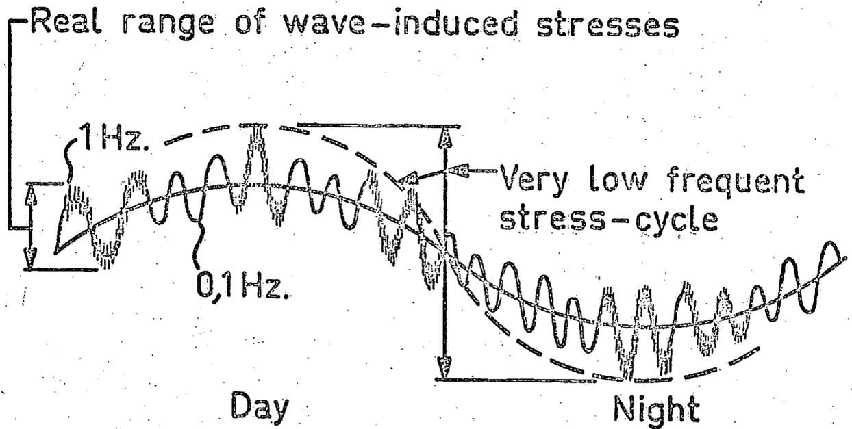
FIG.2 COMPONENTS OF STRESSES.
