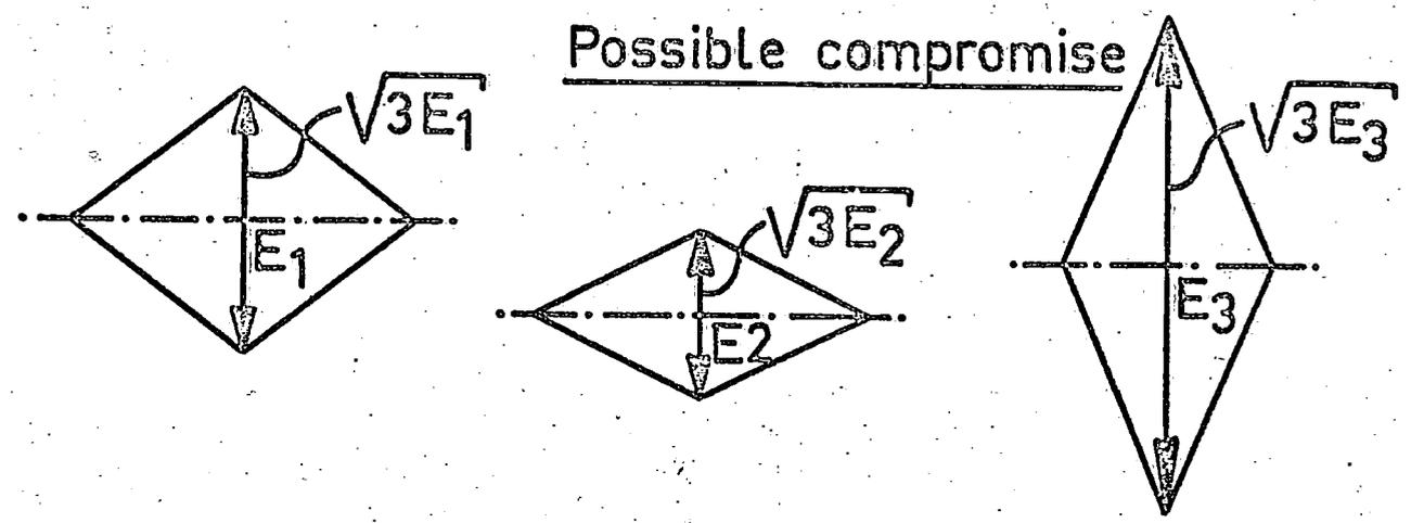
FIG.3 POSSIBLE SIMPLIFICATION OF RECORDS OF WAVE INDUCED STRESSES.
